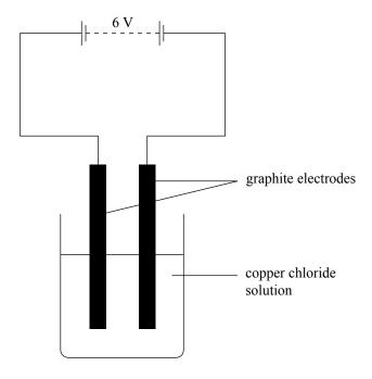
During this electrolysis, a student noticed that copper metal was deposited at the cathode and chlorine gas was given off at the anode.
